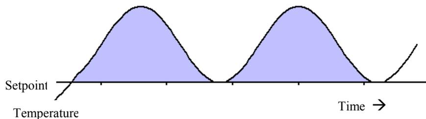
In the case described above, the SCR controlled heater would modulate the heater to supply 50% heat output to satisfy the zone. This results in a more consistent discharge temperature and therefore a more comfortable zone, without the wasted energy.
