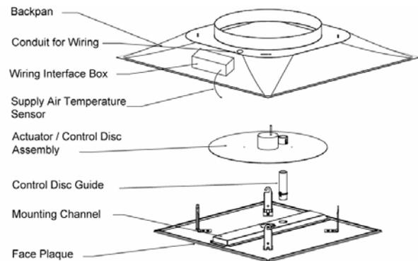
Master diffusers are created by connecting the T<sub>3</sub>SQ -1 diffuser to a wall mounted controller / thermostat using the blue RJ-45 control cable. T<sub>3</sub>SQ-1 drone diffusers are created by connecting the diffuser to a master unit using the blue RJ-45 control cable.
